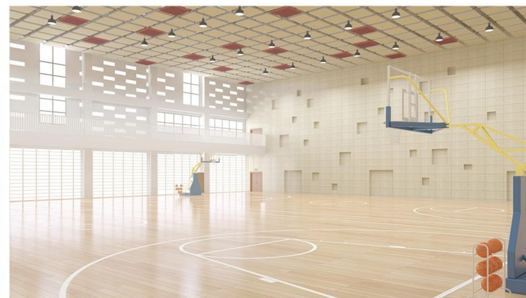
Type:E-shape hole E5/1.5 Perforation rate:7.0%
