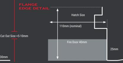
Fire Rated Hatches can be designed for custom sizes but cannot exceed and are limited to a maximum size. Specifications will change as sizes increase.
