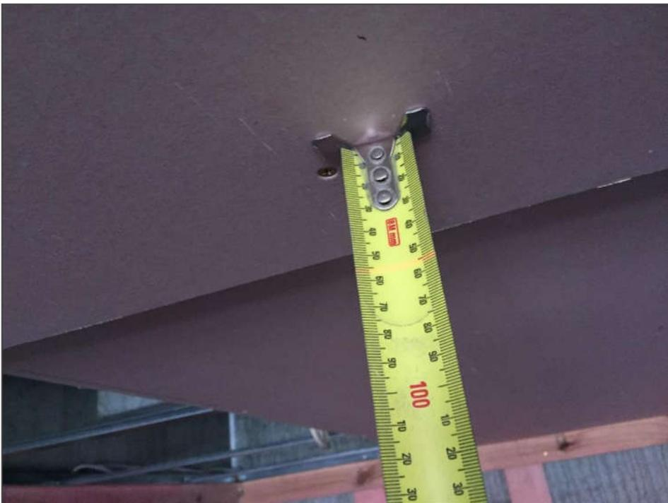
Figure 8: 16mm Plasterboard Grid System - Deflection measurement (2) for three layers of GIB
