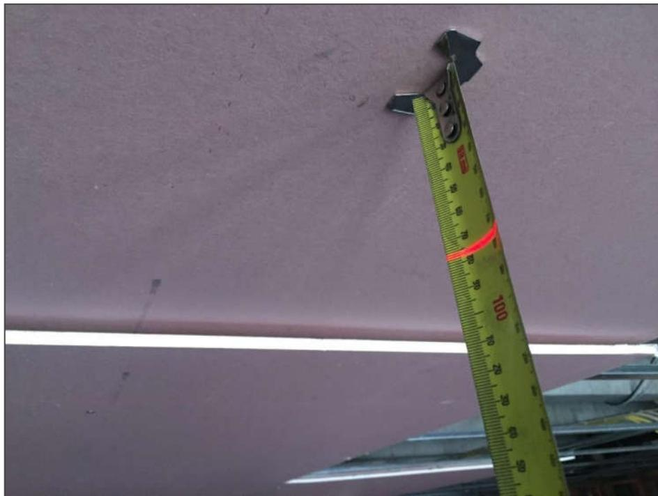
Figure 6: 16mm Plasterboard Grid System - Reference measurement for final deflection check
