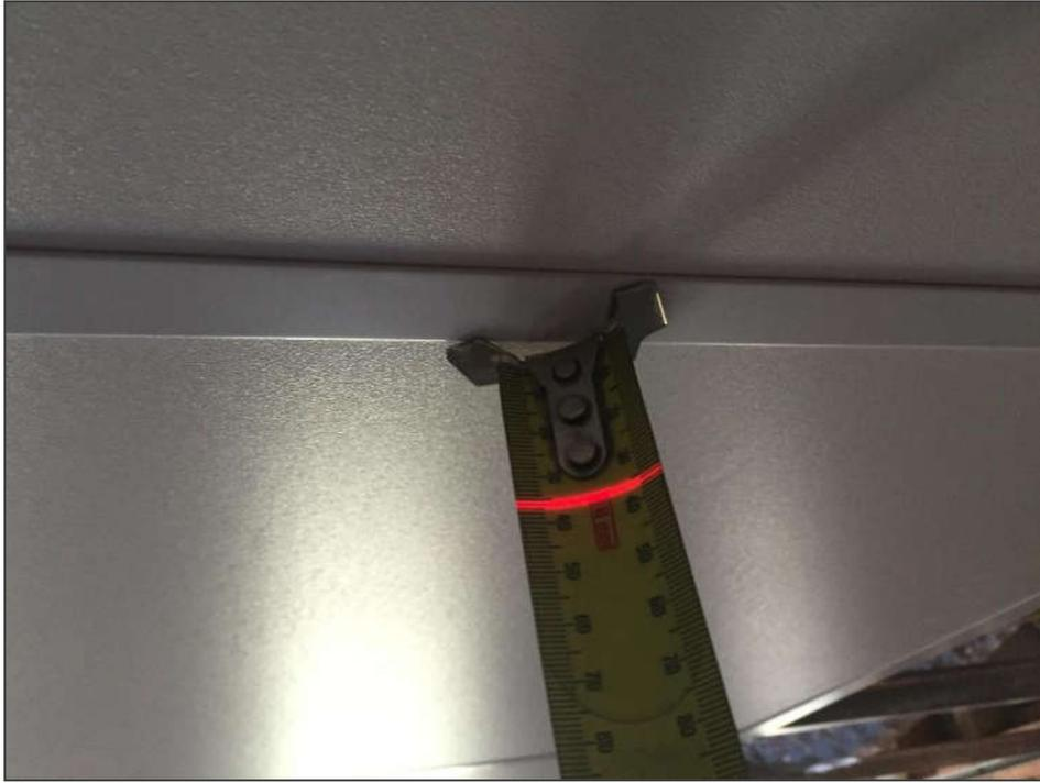
Figure 3: Ecoplus Fastlock System - Example of measurement for deflection
