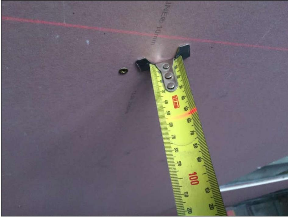
Figure 7: 16mm Plasterboard Grid System - Deflection measurement (1) for three layers of GIB
