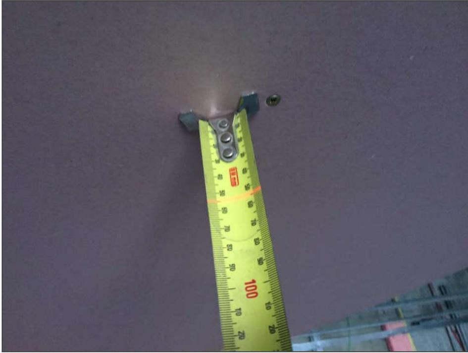
Figure 9: 16mm Plasterboard Grid System - Deflection measurement (3) for three layers of GIB
